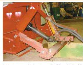
Home-built 3-pt. hitch pins onto snowblower's factory 3-pt. brackets. Lower "push arms" bolt onto a steel plate that fits under tractor's drawbar.
