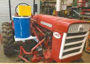
to get off the tractor." Myers says it only takes about 5 min. to put the bracket on, and by unbolting the ring he can quickly remove the motor and gearbox for access to the paddles and gate valve. He mounted a battery bracket on the other side of the tractor in case he ever needs to use the tractor's battery for something else.
