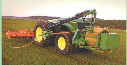
Deere's prototype self-driving electric tractor runs off 300 kW power, which is supplied by a cable that remains connected to tractor as it works its way across fields.
