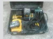
case to make room for the chargers, which are held in place by a zip tie. The lid can be closed with the batteries hooked up to the 3 chargers. The chargers plug into a 3-way
