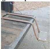
Bent straps on add-on step slip over tailgate.
