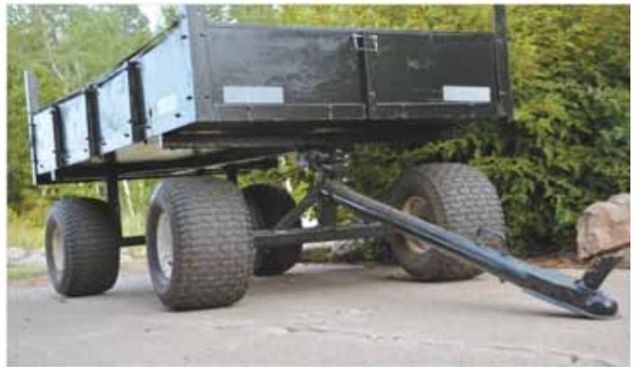
**LeRoy Momper wanted an ATV wagon with a shorter turning radius, so he built one that allows the front axle to swivel 360 degrees.**
