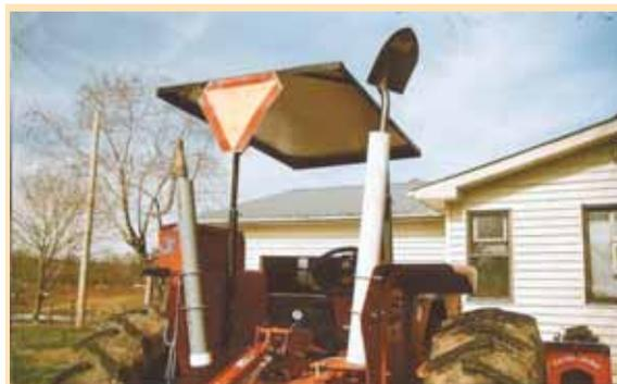
**Pvc tool holders U-bolted to tractor fenders make it easy to carry various long-handled tools.**
