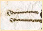
Lawrence converted a grab hook chain to a slip hook chain by cutting off the top 1 ft. of a slip hook chain and slipping the bottom link onto the grab hook.
