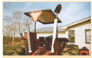
Pvc tool holders U-bolted to tractor fenders make it easy to carry various longhandled tools.
