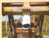
Lawrence uses short piece of pipe welded to bottom of bale spear to push metal fence posts into the ground.
