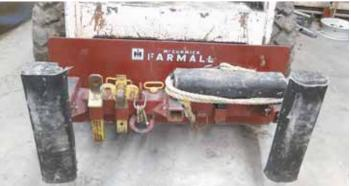
"Everything" toolbar is fitted with receiver hitches, straight hitches, ball hitches, pintle and clevis hitches, chain hooks, and push bars.
