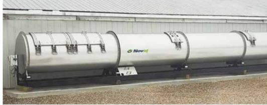
A 1/2 hp. electric motor rotates the big composter in 15 to 20-min. cycles 6 to 12 times a day, turning carcasses into compost in 7 to 10 days
