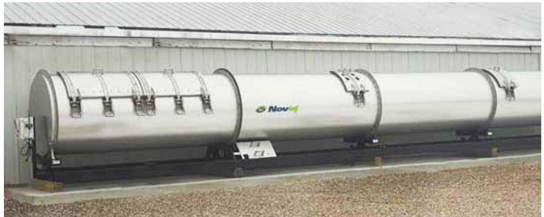
A 1/2 hp. electric motor rotates the big composter in 15 to 20-min. cycles 6 to 12 times a day, turning carcasses into compost in 7 to 10 days.
