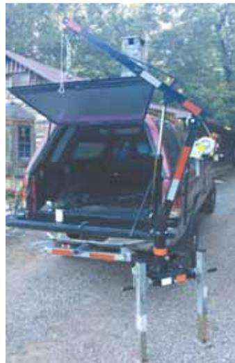
Boom lift fits into 1 of 3 receiver hitches on rear-mounted toolbar. McMahon also uses receiver tubes in his shop by attaching them to metal poles.
