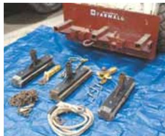
Photo shows the skid steer-mounted toolbar with all attachments removed.
