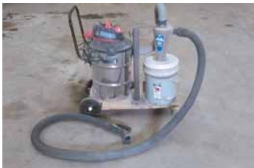
Dale McLaen added a cyclone-type dust separator to a new heavy-duty shop vac in order to catch fine dust before it can reach the filter.
