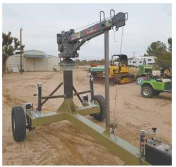
Kurt Carlson converted an old Venturo truck-mounted crane into a 2-wheeled model that hooks up to a pickup or ATV.
