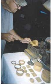
James White turned a grinder into a lathe by welding a nut onto the grinder shaft, and then screwing a 4-in, faceplate onto it.
