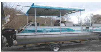
Plunkett replaced the small vinyl roof on his pontoon boat with a bigger one made from sheet metal siding.
