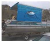
Roll-up vinyl sides drop down to convert pontoon into a camper.
