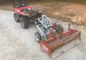
Home-built, 3-pt. tool carrier rides on a pair of 8-in. wheels. A remotecontrolled electric winch is used to raise and lower the implement.
