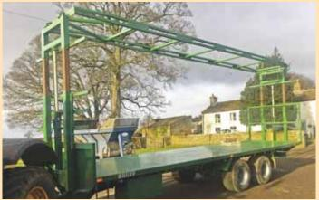
Hydraulically-controlled cage on trailer clamps down on top of bales once they're loaded, eliminating the need to strap them down.
