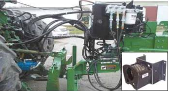
Pto-powered HydraBoost pump is designed to meet the needs of new planters and other hydraulic power hogs. PumpDoctor bracket, lower right, secures pto pump to reduce vibration.
