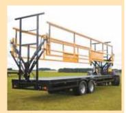
Hydraulic-operated, retractable sides hold bales in place.
