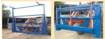
When he picks up a pile of square bales, Tucker can use the hydraulic-controlled top frame to hold them in place. Spikes fold up flat when not in use.
