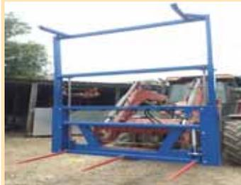
When he picks up a pile of square bales, Tucker can use the hydraulic-controlled top frame to hold them in place. Spikes fold up flat when not in use.
