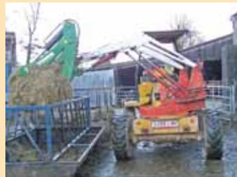
Pivoting loader makes it possible to reach into bunks when feeding livestock.
