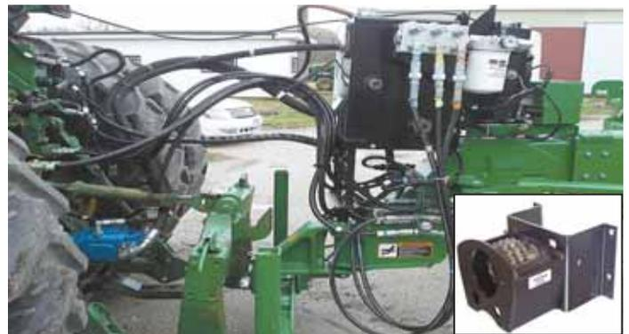
Pto-powered HydraBoost pump is designed to meet the needs of new planters and other hydraulic power hogs. PumpDoctor bracket, lower right, secures pto pump to reduce vibration.
