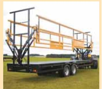
Hydraulic-operated, retractable sides hold bales in place.
