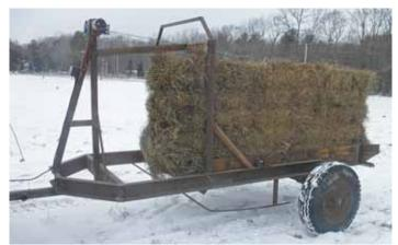
Big bale trailer uses an electric winch and hook to pull bale onto trailer. Wilson spreads flakes by pulling bale forward through an overhead arch fitted with "flake retainers".
