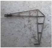
Bale hook is a right angle device reinforced with roof truss-like supports.
