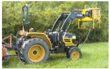
Loader-mounted fuel tank is gravity fed, with no extra cost for a pump.
