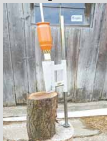
Sliding hammer (orange) slams down onto splitting head to chop logs. A smaller blade between axe head and rod cuts up kindling.
