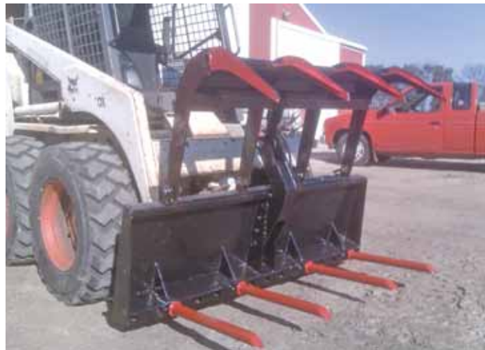
McLae removed the teeth from an old manure grapple fork, then welded steel tubing supports in place and slipped 1 7/8-in. high strength steel teeth into them.
