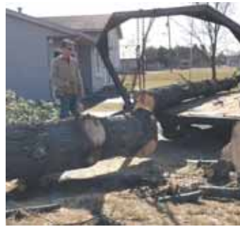
Matt Eby loads logs onto rebuilt flatbed trailer using a 12,000-lb. winch connected to a pivoting steel arch. Log is chained to arch (left) and then arch is winched upright and forward to pull log onto trailer. A steel retainer and spring shock pin attach to both sides of arch.
