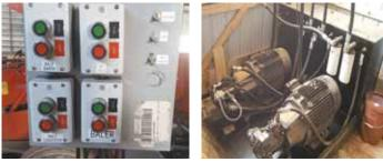
Control panel is located in center of U near baler (left). Bale Converter and Bale Baron operate on hydraulic pumps powered by two 3-phase electric motors
