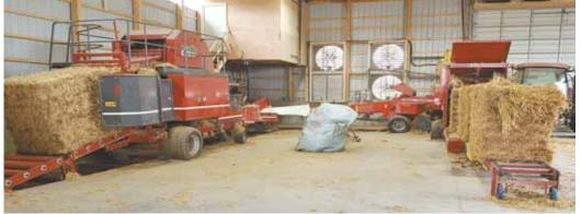
Boll converts big square bales into small bales, which are then compressed into 21-bale packs for shipping. U-shaped setup includes Bale Converter at right, baler at center, and Bale Baron 21-Pack at left.
