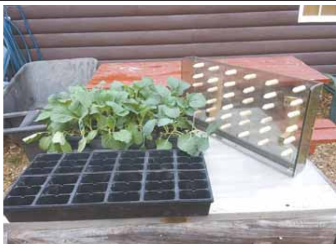
User grabs a pair of handles and presses board down onto tray, with the pegs forming a hole in the soil in each cell.
