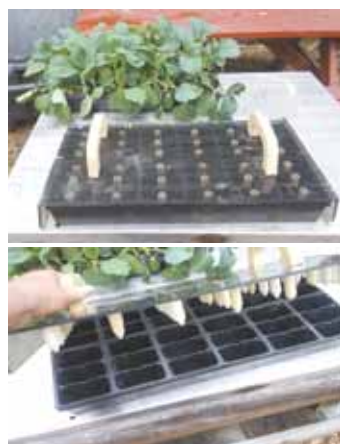
"Dimple board" consists of 36 wooden pegs set in rows and screwed to a sheet of Lexan.
