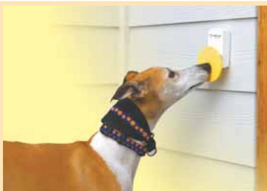
Dog uses its nose to nudge round “push plate” attached to transmitter. It activates a receiver, which sounds a chime inside the house.
