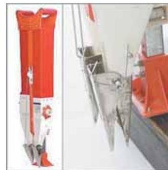
Stand up planter comes with spring-loaded tips (right) and has 2 halves, one for dispensing seed and the other for fertilizer.
