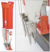
Stand up planter comes with spring-loaded tips (right) and has 2 halves, one for dispensing seed and the other for fertilizer.
