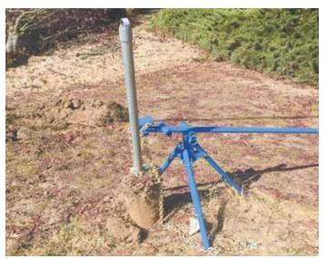
"The 3 legs pull straight up from the load, which provides amazing power," says Rowdy Sloggett. Leverage can be adjusted by moving handle forward and back, and snugging up the chain.
