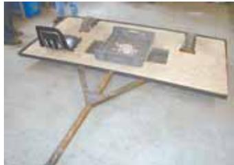
Redesigned planter has adjustable wheels mounted on a rear-mounted toolbar, which can also hold tools such as hilling discs.
