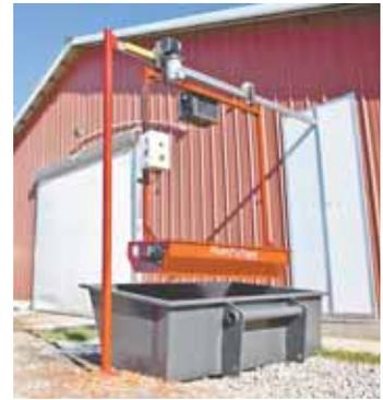
The trolley on rails is available in battery-powered models with either dumping or fixed trays.
