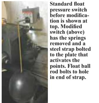
Standard float pressure switch before modification is shown at top. Modified switch (above) has the springs removed and a steel strap bolted to the plate that activates the points. Float ball rod bolts to hole in end of strap.
