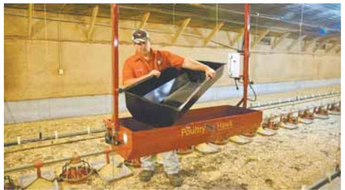
Poultry Hawk was developed to move dead birds out of poultry houses, but it's being used with feed trays, egg carts and even a sprayer for applying vaccines, insecticides and disinfectants.
