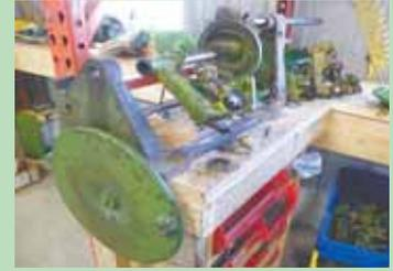
**Green Baler Parts specializes in repairing and rebuilding Deere small square baler parts. Photos show bale knotter frame (left) and knotter rebuilding equipment.**
