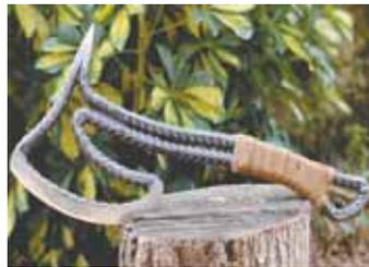
**Rebar hatchet (above) has a sharp blade on one side and a pointed awl on the other. Bigunas also used rebar to make this big C-clamp.**
