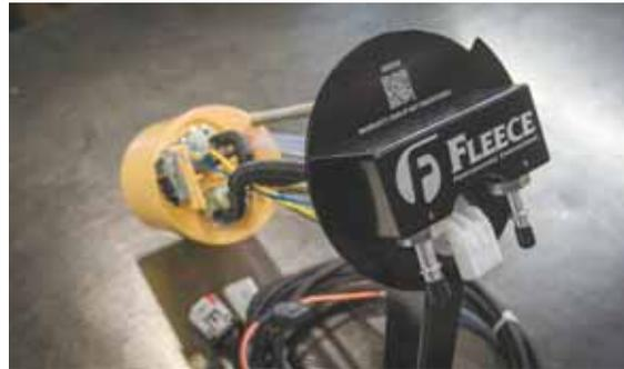
**Drop-in PowerFlo lift pump is designed for Dodge Cummins diesel engines, providing more fuel exactly when the engine needs it.**
