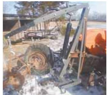
**Rice welded a length of channel iron to the back of the lift and then welded on short pieces on either side to form a 3-pt. hitch.**
