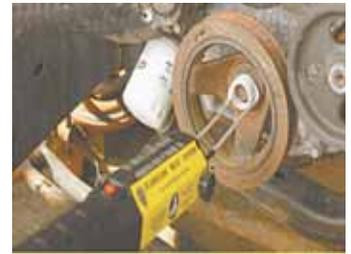
**Mini-Ductor tool heats up nuts or bolts so they can be safely removed, without the dangers of an open flame.**
