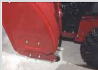
**Hugo Bach, Osoyoos, B.C.:** He replaced the metal skid shoes on his walk-behind snowblower with wheeled “runners” that won’t wear out like skid shoes do. He removed the skid shoes and their slotted mounting brackets from the snowblower
