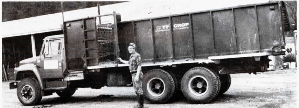
Schrauwen spent $55,000 to equip his truck to do a variety of jobs. Side unload door, above right, feeds into bunks.
