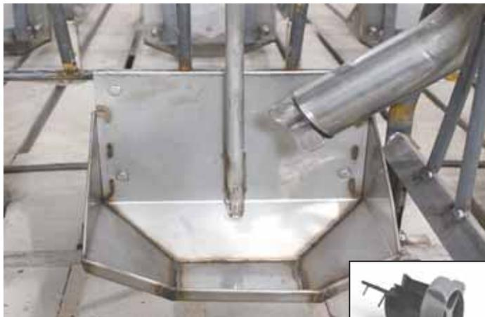
Hogs spin wheel on "Meal Meter" to drop feed down into the trough.
