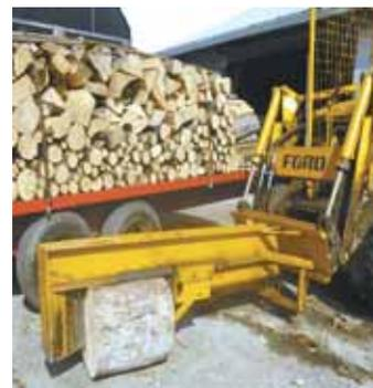
Log splitter is built from 2 pieces of channel iron mounted back to back, with a "window" in between. It can handle wood chunks from 4 to 20 in. in diameter.
