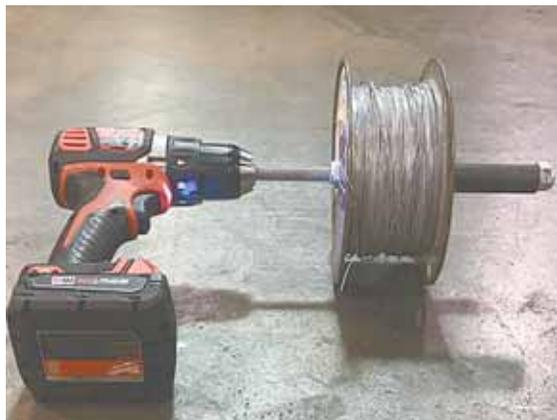
Cordless drill with a 12-in. length of all-thread rod runs through wire spool to roll up wire.
