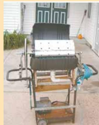
Electric motor belt-drives round metal tumbler to scale up to 50 fish at a time.
