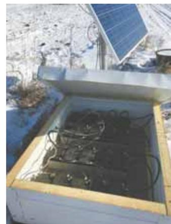
Solar panels stand next to insulated chest that holds the batteries shown above. Cattle drink through 10-in. dia. hole in aluminum cap, shown at left.
