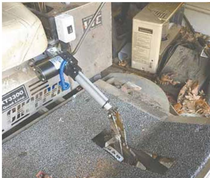
Ed Clayton wanted to raise the deck on his zero-turn mower without having to push hard on the pedal, so he replaced it with an actuator kit mounted below the seat.
