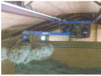
Wet hay is hauled from the field to a specially designed building with drying space, where it's picked up by a grapple that travels on rails. Crane has a cab for the operator.
