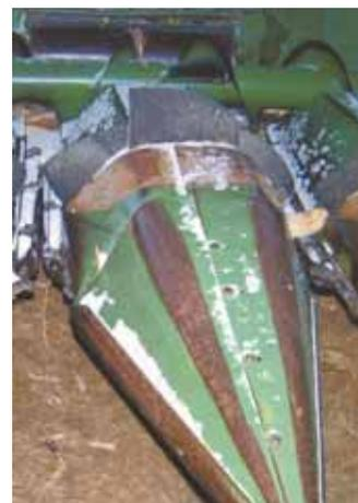
Short lengths of conveyor belting bolted onto snouts keep ears of corn from falling to the ground.
