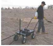
Engine exhaust goes into a patented resonance chamber that mutes the sound and feeds both hoses.
