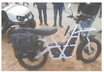
New 2-WD scooter has an electric motor in each wheel, and a big lithium ion battery that can also be used as a mobile power station. It has a 75-mile range.
