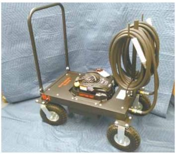
"It's a simple, safe way to kill gophers and works fast," says Bill Enderson. His 4-wheeled machine comes with two 25-ft. hoses that pump out carbon monoxide.
