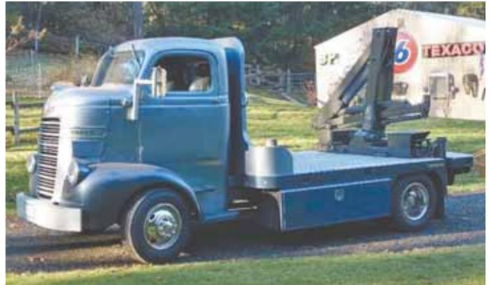
**Charlie Brown converted an old Dodge COE semi truck into this shop truck complete with a flatbed and knuckle boom crane.**
