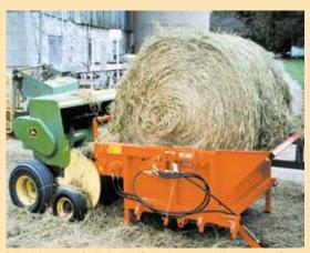
Machine unwinds bale directly over pickup reel of any small square baler. You can see a video of the Altec bale unwinder at our YouTube channel: "thestgeorgeco".
