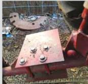
U-shaped steel plate bolts onto 3-pt. lower lift arm, making it safer to climb up onto tractor.
