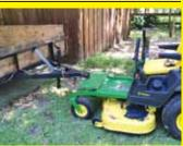
I used 3/8-in. all-thread rods to bolt a 1 by 2-ft. board on front of my Deere ZTrak mower and mounted a 16-gal. spray tank on top of it. It lets me use a wand to spray insecticide on my pecan trees right from the mower seat, which is a lot easier than walking around with a backpack sprayer. A pair of bolt-on metal brackets, one at each end of the board, help support the tank's weight. A pair of rubber straps with S hooks are used to attach the tank to holes drilled
