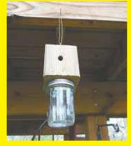
My dad and I built a 4-sided carpenter bee trap by screwing a canning jar to the bottom of a box made from 7-in. long pieces of wood. We drilled 1/2-in. holes into all sides of the box at an upward 45-degree angle, which prevents direct sunlight from shining in. We also drilled a 1-in. hole in the bottom of the box and screwed the jar on over it. The box hangs from a wire attached to our barn.
