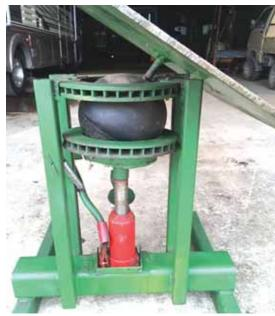
Bowling ball serves as a pivot point, allowing welding table to be easily tilted or rotated.
