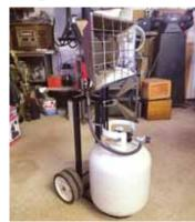
Home-built hand cart makes portable propane heater easy to move around.
