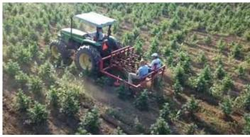
Ride-on "Hemp Hawk" provides manual control of hydraulic-powered cultivation in hemp fields. Each operator uses hand grips to control 2 sets of 10-in. dia. spinning cultivator heads
