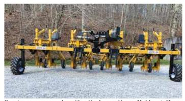
Operators can remove weeds on either side of row, and in-row. Models up to 12 rows wide are available.
