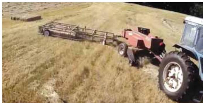
The 10-bale Hay Accumulator turns 2 bales sideways, then adds 2 sets of 4 bales lengthwise. Alternating the 2 odd bales makes trailer load more stable.
