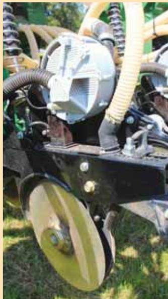
and there are LED sensors in the seed tubes so he can monitor accuracy while planting. He's used the planter both for corn and canola seed.
