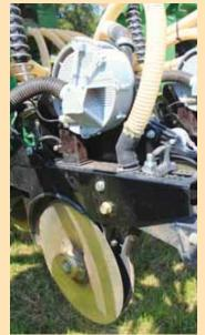
and there are LED sensors in the seed tubes so he can monitor accuracy while planting. He's used the planter both for corn and canola seed.
