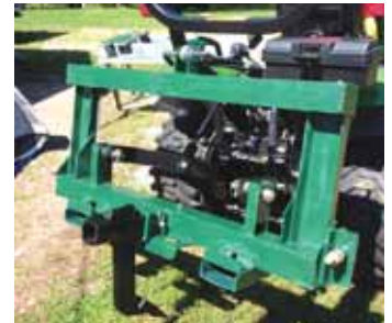
Frame can also be used on the 3-pt. hitch at back of tractor. Here frame is used with a “vertical ripper” that can dig narrow trenches up to 1 ft. deep.
