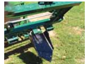
Receiver hitch-mounted V-shaped “shovel” can dig 2 ft. down to remove rocks or to make holes for planting trees.
