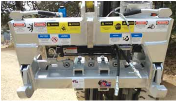
“Our Camera Guided Hitch can side shift a 3-pt. implement to provide precise control. It works at speeds up to 4 mph,” says Ryan Herbon, Agmechtronix.
