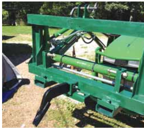
Loader-mounted steel frame has a pair of slots for forks and a receiver hitch in the middle. “Horizontal ripper” shown in photo is used to dig out rocks and tree roots.
