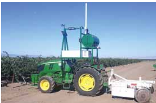
This tractor was converted to spray fruit and nut trees in California. Seat and steering wheel were replaced by high definition cameras, and a large diesel tank was added for additional range.
