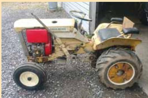
Repowering older gas-powered tractors with diesel engines is the answer to poor quality gasoline, which is often the cause of engine problems, says Jim VanDerEems. He specializes in Allis Chalmers tractors.
