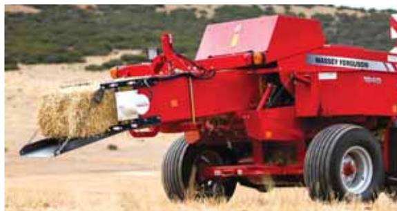
Microwave technology is used to measure hay moisture as bale exits bale chamber. Models are available for both big and small square balers.
