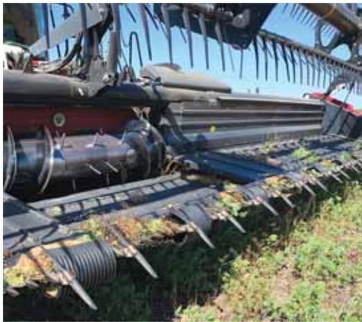
To keep from damaging his soybeans while harvesting the camelina cover crop, Joe Breker installed pieces of drain tile on his combine header to push soybean rows below cutterbar.
