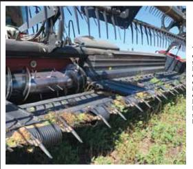
To keep from damaging his soybeans while harvesting the camelina cover crop, Joe Breker installed pieces of drain tile on his combine header to push soybean rows below cutterbar.
