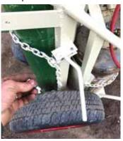
A spring-loaded, over-center chain holds oxygen tank in place in the vertical position.
