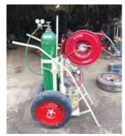
Big car wheels and a balanced design make home-built torch cart easy to move around the shop. Note 50-ft. hose reel.
