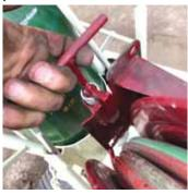
Spring-loaded T-bar rides in a slot on hose reel hinge plate to hold reel in place.
